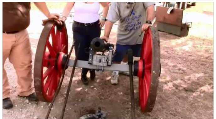
The tube had an unusual touch hole. It was a hollow pipe for introducing touch powder or a fuse into the tube
